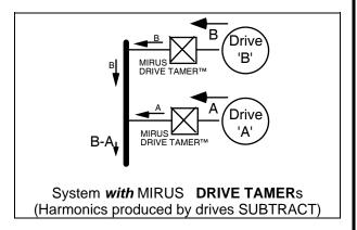
The **MIRUS** DRIVE TAMER<sup>™</sup> approach has none of the risks that installing capacitors or tuned filters are known to have in low-voltage systems, including the risk of resonance and overloading of
