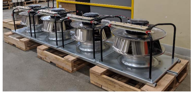
Fig. 14 Array of 4 x 3.75 HP EC fans during factory testing
