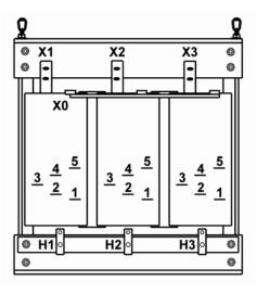
Figure 3-1 Transformer Taps, accessed from front of HMPC
