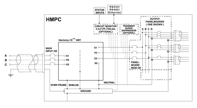
Figure 2-6 Grounding Within the HMPC Electrical Path
