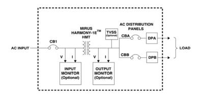
Single –line diagram of HMPC-084 with Harmony-1E<sup>™</sup> HMT Figure 1-4
