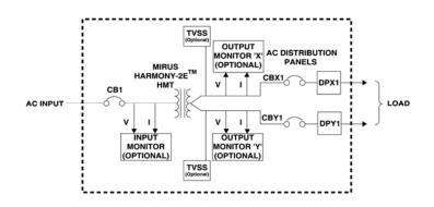
Single –line diagram of HMPC-084 with Harmony-2E<sup>™</sup> HMT Figure 1-5
