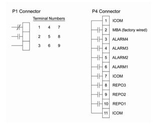
Figure 1-8 Summary Alarm Connections (P1) / Alarm and REPO I/P Connections (P4)
