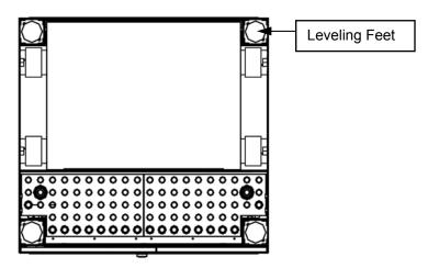
Figure 2-3 HMPC Bottom View showing leveling feet
