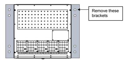
Figure 2-1 Removing HMPC from the pallet (Top View shown)
