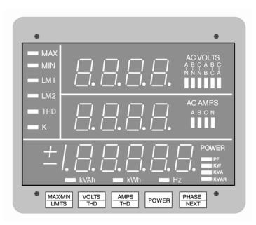
Figure 1-10 Power Monitor Front Panel
