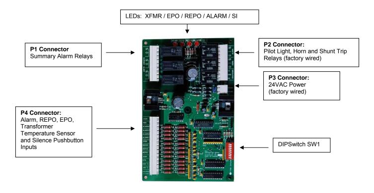
Figure 1-9 Printed Circuit Board detail
