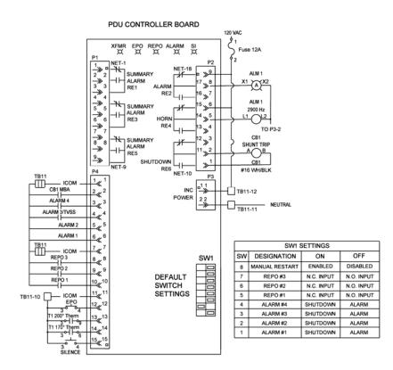
Figure 1-7 PDU Controller Board Layout / DIP SW Settings (SW1)
