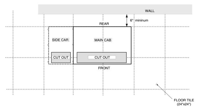
Figure 2-5 Placement, Showing Floor Tile Cut-Outs
