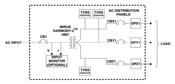
Single –line diagram of HMPC-126 or HMPC-252 with Harmony-3E<sup>™</sup> HMT Figure 1-6
