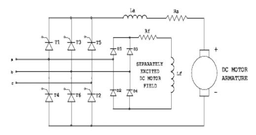
Fig. 3. Typical dc drive and motor schematic.
