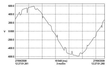
Fig. 15. Voltage notching on supply bus with filter installed.
