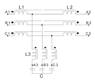
Fig. 8. WSHF schematic [5].
