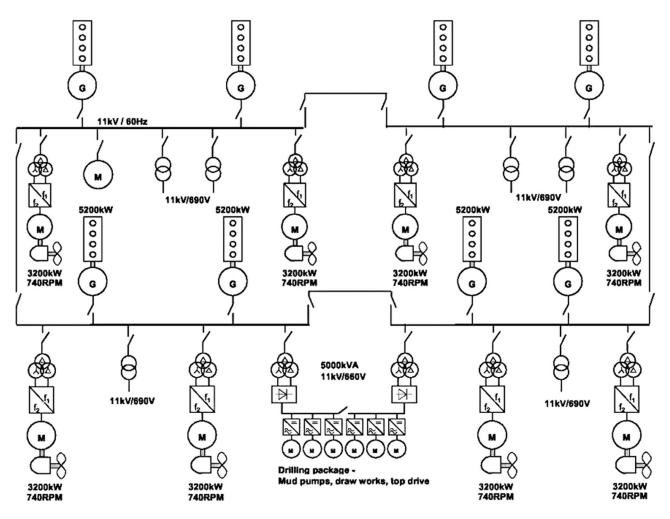
Fig. 2. Typical power system single-line diagram for dynamically positioned Class 3 drilling rig.
