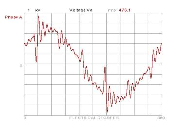
Fig. 9. Computer-simulated voltage at the distribution panel supplying a large dc drive fed from a generator.
