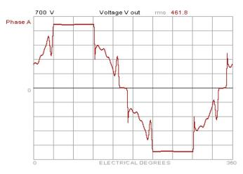
Fig. 10. Computer-simulated voltage at the input to the ac drive with input voltage to the WSHF as in Fig. 9.
