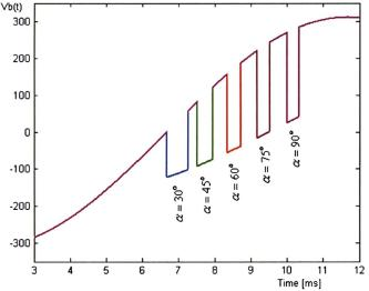
Fig. 6. Notch-depth variations on firing-angle changes [4].
