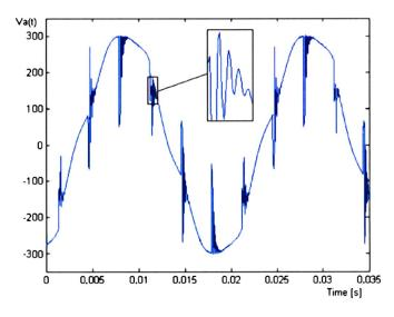
Fig. 7. Commutation notches associated with the operation of an SCR with  $\alpha=45^\circ$  [4].
