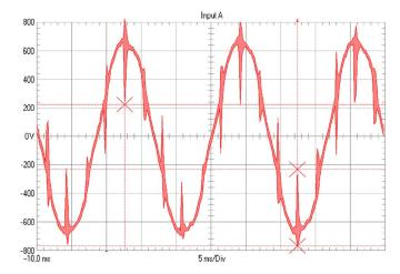
Fig. 1. Drilling-rig voltage waveform with commutation notches and voltage ringing.
