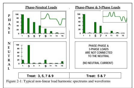
$9^{\text{th}}$  harmonic currents unless their voltage supply is unbalanced. Their principle harmonics are the  $5^{\text{th}}$  and  $7^{\text{th}}$  with  $11^{\text{th}}$  and  $13^{\text{th}}$  also present. They cannot produce neutral current because they are not connected to the neutral conductor. The rectifiers of variable speed drives and Uninterruptible Power Supplies (UPS) are typical examples of three-phase rectifier loads.
