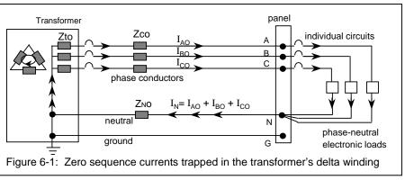
characteristics when significant amounts of 3rd harmonic (and other zero sequence currents) are present on the load side. These harmonics return along the neutral conductor and are trapped in the primary DELTA winding where they circulate causing significant extra heating. They do not flow through to the primary system, but they also are NOT cancelled (Figure 6-1).
