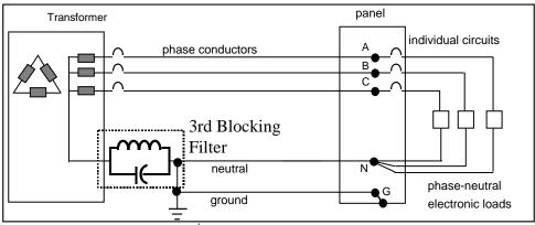
Figure 14: Typical installation of 3rd Harmonic Blocking Filter
