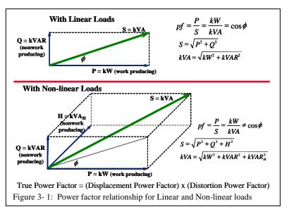
and lower the PF. Inductive loads such as induction motors cause their current to lag the voltage, capacitors cause their current to lead the voltage, and purely resistive loads draw their current in-phase with the voltage. For circuits with strictly linear loads (a rare situation) simple capacitor banks may be added to the system to improve a lagging power factor due to induction motors or other lagging loads.
