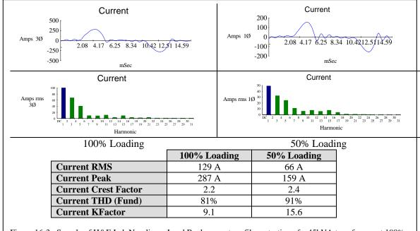
Figure 16-3: Sample of H&E Lab Non-linear Load Bank current profile on testing of a 45kVA transformer at 100% and 50% loading.
