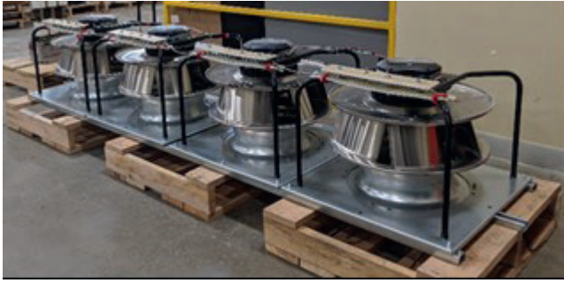
Fig. 11: Array of 4 × 3.75 HP EC Fans during Factory Testing
