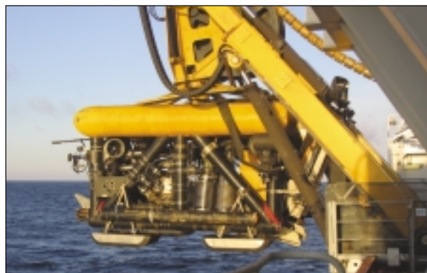
The vessel's PT1 remotely operated vehicle has ten 30kW thrusters and four 300kW pumps.
