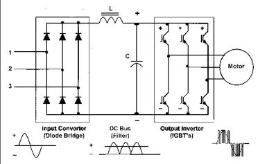
Figure 4-1: Typical Schematic of a PWM Variable Frequency Drive
