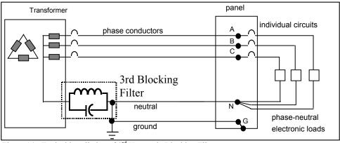
Figure 14: Typical installation of 3<sup>rd</sup> Harmonic Blocking Filter
